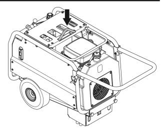
Make sure no one is standing under the hydraulic unit if it has to be moved by hand up into or off a trailer or up and down a slope.
