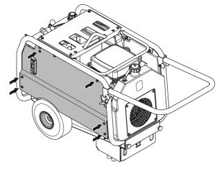
Remove the side panel to access the oil plug and the oil filter
